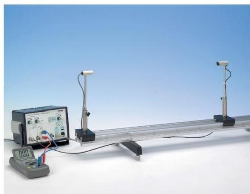
Figure 1 Measurement kit for checking the law of absorption of ultrasound in the air
